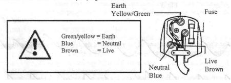
As the colours of the wires in the mains lead may not correspond with the coloured markings identifying the terminals in your plug, proceed as follows.
